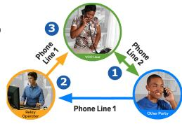
While the 1st phone line is connected to the Relay Operator, the VCO user speaks directly to the other party on the 2nd phone line. (1)
